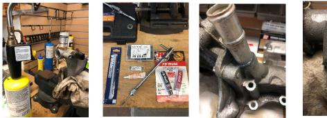
15. After the coolant fittings were back on the engine, I decided to deal with the sparks and coils. All was well until the coil for cylinder 6. The coils are the new style and there is no clearance between the VTG activators and the coil, so some filing is needed (or you can get the old-style coil).
