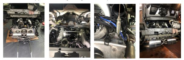
25. With the engine back in, I hooked up the remaining coolant lines, reinstalled the PS pump and finished up the rest of the connections for fuel, hydraulics and electric. I used a Schwabben coolant fill too to create negative pressure and suck in the new coolant. I also use a mix of 4 0-40 and 5 5-50 synthetic for oil and was able to use my new dipstick to check the level without starting and warming up the engine. I used Pentosin for the PS system. Oil and hydraulic fluid are from Red Line.
